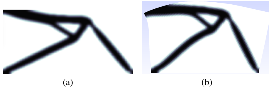
Figure 15 – Inverter mechanism for the static case: (a) undeformed and (b) deformation mode of the first natural frequency.
