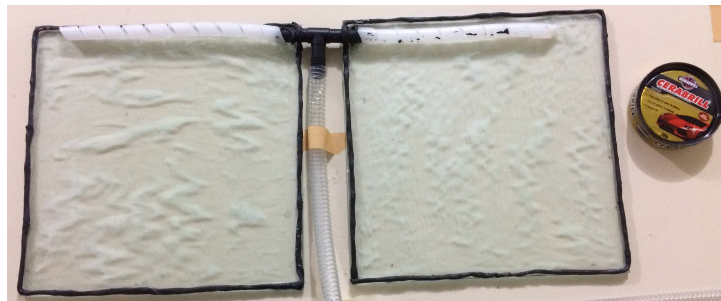
Figure 4.2 – VARTM manufacturing process: step 1.
