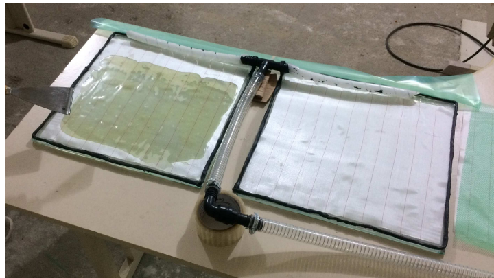
Figure 4.4 – VARTM manufacturing process: step 3.
