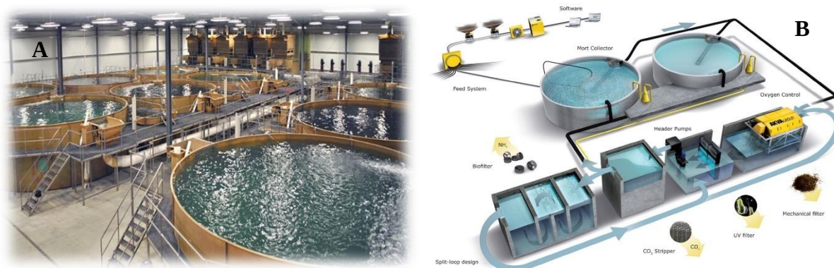
Figura 4. Recirculating aquaculture system “RAS”
